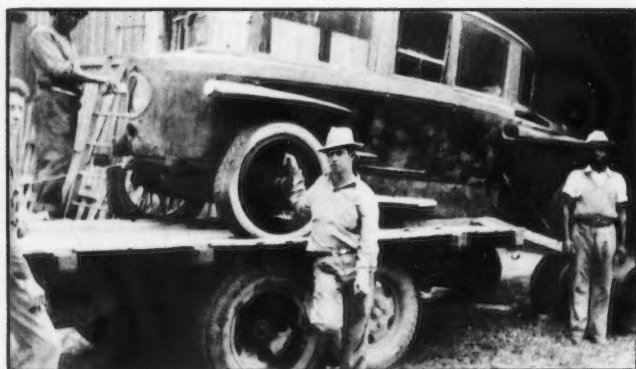
HERE'S ONE FOR YOU --- A RUMPLER, MADE IN BERLIN, GERMANY. IT HAS A REAR ENGINE 4 CYLINDER MOTOR. OWNED BY C. R. TYDINGS, OF OCALA, FLORIDA.
